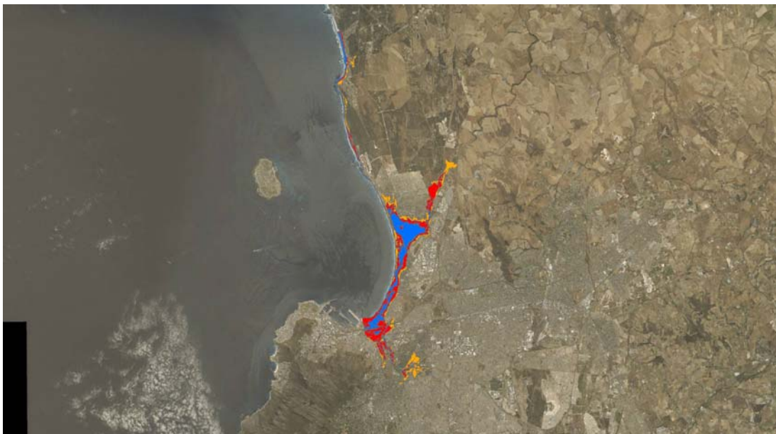
Figure 6: Aerial photograph of the coastline Melkbos to the port showing the inundation that would be caused by a 2.5 (blue), 4.5 (red) and a 6.5 (orange) sea-level rise event.
