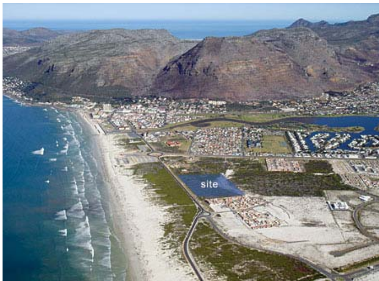
Figure 14: This photograph of a proposed up-market development site on the False Bay coast (not between Melkbos and the Port) shows the exposure of much coastal development to sea-level rise events. The photo also shows the vulnerability of Baden Powell Drive (road in foreground) and the importance of the beach sand, dune cordon and dune vegetation as a natural sea-level rise buffer.
