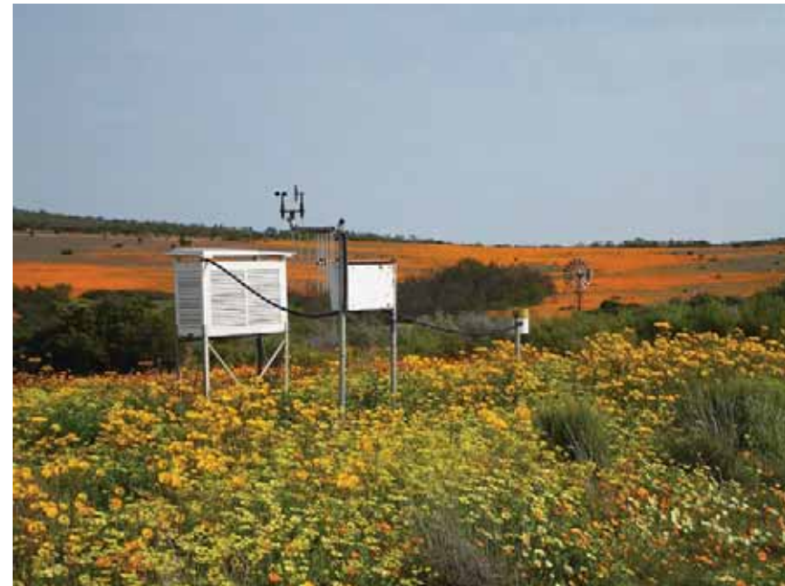
Figure 1.22 An ARC Automatic Weather Station, Western Cape. [Reproduced with permission: ARC, Pretoria]
