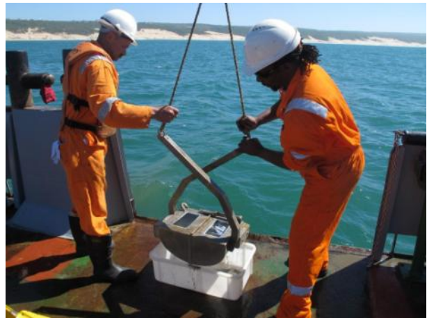
D) SMIT Amandla vessel crew assisting with retrieval of the Van Veen grab to obtain a macrofauna sample
