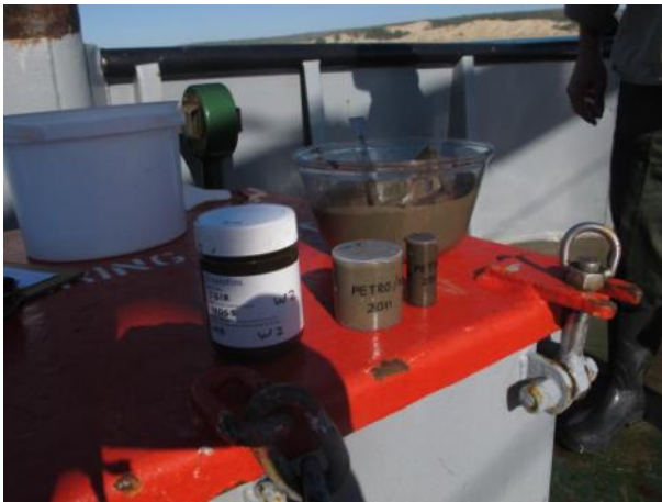
C) Various containers prepared for different sediment property analyses: grain size, organic carbon, hydrocarbons and metals
